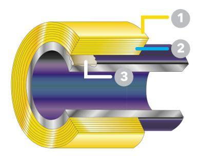
**Clock Spring**<sup>®</sup> is used to repair corrosion defects with up to 80% metal loss, as well as mechanical and third party damage. The repair is stronger than the pristine pipe allowing the pipeline to be returned to service at 100% of its maximum allowable operating pressure.
