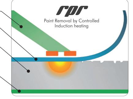
The induction disbonder works by the principle of induction. Heat is generated in the steel substrate and the bonding is broken. The coating is then removed entirely without disintegrating and completely free from contaminating agents, i.e. blast media.
