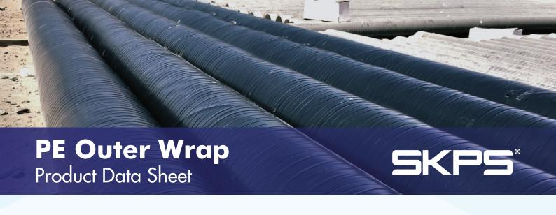
Viscotaq® PE Outer Wrap is a Heavy Duty polyethylene backing in the form of a roll, calendered with an adhesive. The tape is used as an Outer Wrap for the mechanical protection of Viscotag® products against soil stress, back fill procedures and other forms of mechanical impact. Furthermore, it gives a continuous external pressure to the Viscotag® corrosion prevention inner material and accelerates the process of the formation of a homologue continuous inner coating.
