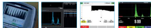
LARGE 3.5" OUTDOOR READABLE DISPLAY CYLINK SOFTWARE B-SCAN WITH AUTO START/ PAUSE/CONTINUE LIVE A-SCAN FOR FURTHER VERIFICATION
